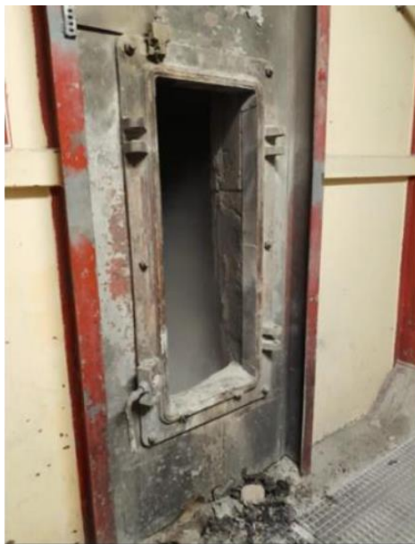
Figure 4 : Access door broken in half due to the explosion
