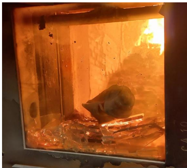
Figure 7 : Broken sight glass after an explosion
