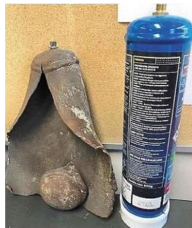
Figure 1 : N2O canister before and after explosion
