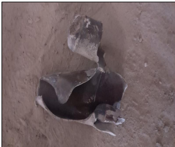
Figure 6 : Exploded nitrous oxide canister found near the fine particle extraction screw
