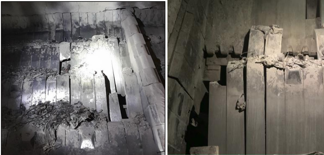
Figure 3 : Broken grate bars
